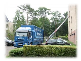
Cranes and external elevators – Oversized items that don't fit into your new property (usually an apartment) will be removed/delivered using an external hoist or crane (whichever best suits the situation).
